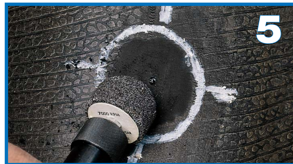
5. Use a low speed buffer (max. 2,500 rpm) and a buffing stone to buff the innerliner 1/2-inch larger than the patch (RMA #1 Buffing Texture.)
