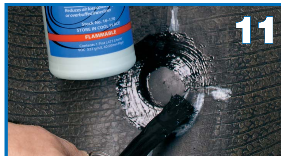
11. Apply repair sealer to the overbuff area.
