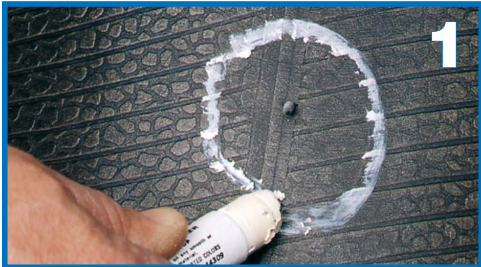
1. Locate injury and circle with a tire crayon. Consult information about reparability of tires and check that the injury is within the tire's repairable area. DO NOT INVERT RADIAL TIRES.
