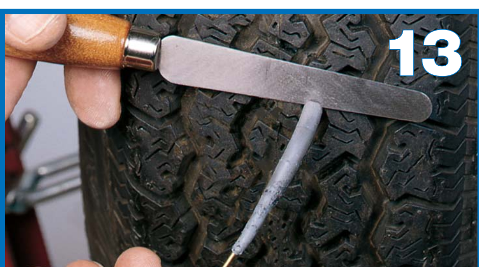
13. After inflating, cut the plug flush with the outside tread area. The tire is now ready to be returned to service.
