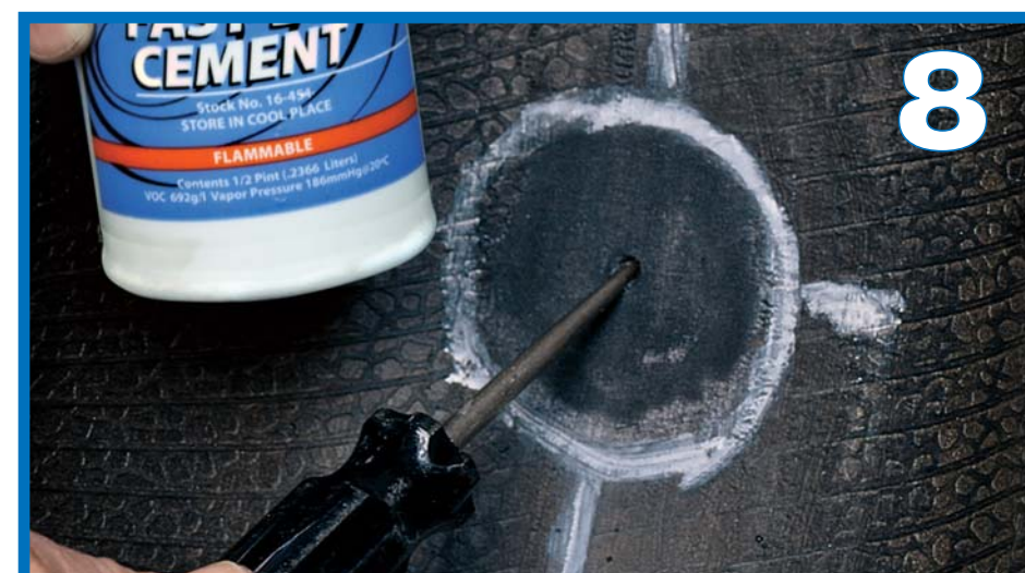
8. Dip awl into cement and insert into injury to lubricate the injury. DO NOT ALLOW CEMENT TO DRY. DO NOT DRIP CEMENT ONTO BUFFED AREA.
