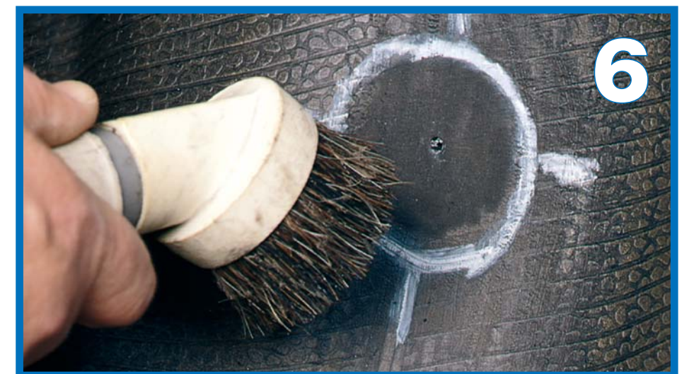
6. Remove buffing dust with a vacuum, then clean the buffed area with cleaner fluid and a scraper to avoid contaminating the injury channel.
