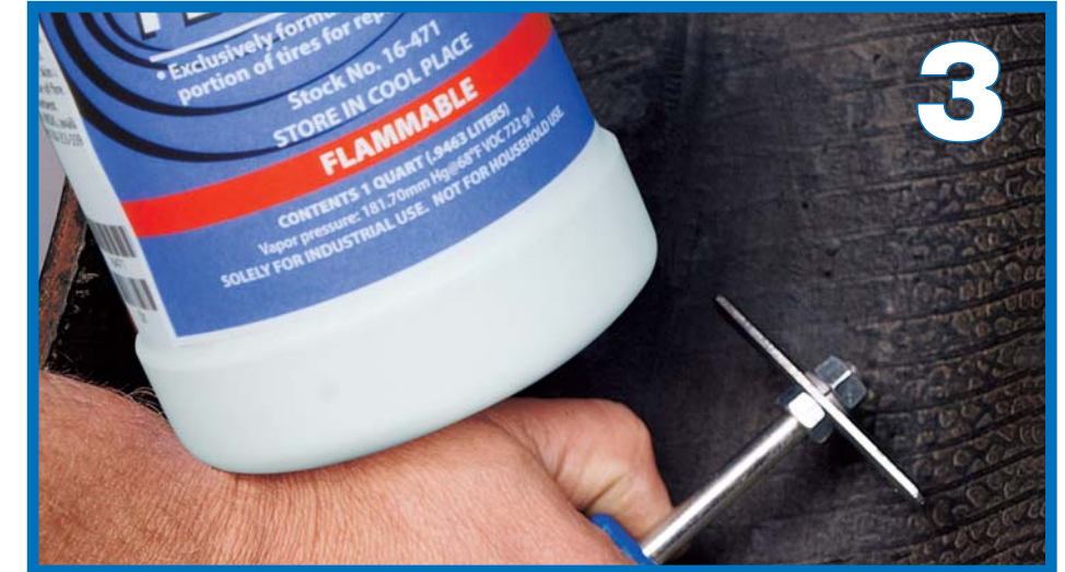
3. Clean the area around the injury with cleaner fluid and a scraper.
