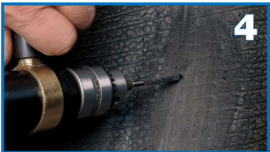
4. Using a low speed drill (500-700 rpm) and the appropriate size carbide cutter, ream the injury following the angle of penetration four times from the inside of the tire, and four times from the outside. Use proper eye protection.
