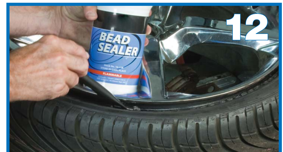
12. Apply bead sealer to the head of the tire before inflation to help prevent air loss around the bead.
