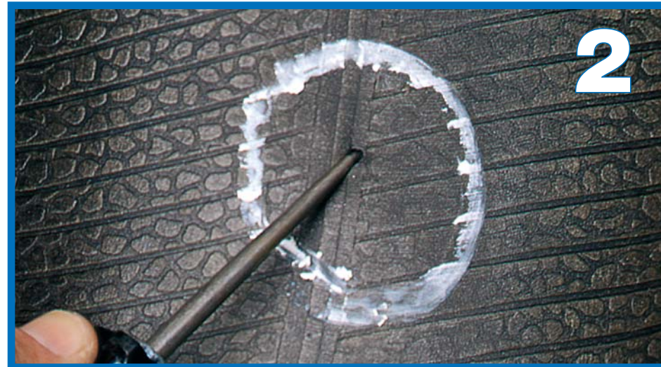
2. Remove the foreign puncturing object and probe the injury with an awl to determine the angle of penetration.
