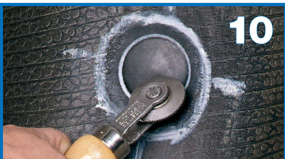
10. Stitch the repair unit vigorously from the center working outwardly. Use as much hand pressure as possible.
